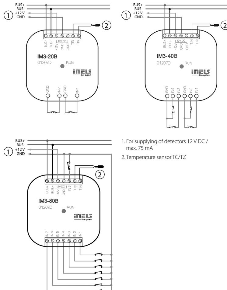
1. For supplying of detectors 12 V DC / max. 75 mA
