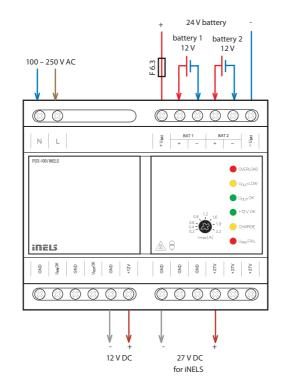
• PS3-100/iNELS is a stabilized switching power supply, with the total
