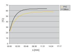
PVC -reaction to water temperature from 22.5 1°C to 58°C. Silicone - reaction to water temperature from 22.5°C to 63.5°C.
