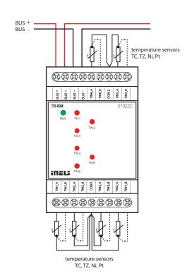
ADC3-60M | Analog-digital converter
