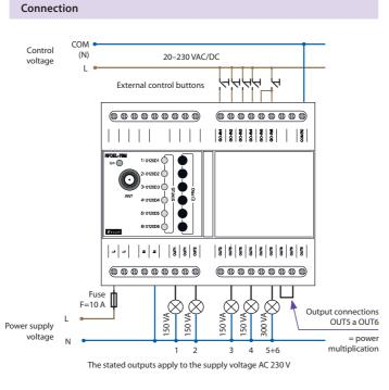
\*Warning: it is not allowed to simultaneously connect loads of inductive and capacitive type in the same channel.
