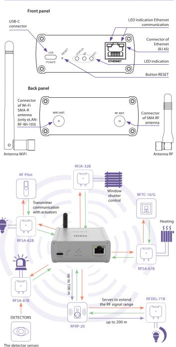
movement and switches on alarm System
