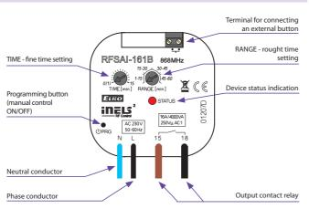
Compatible wireless detectors: Movement: RFMD-100 Door/Window: RFWD-100
