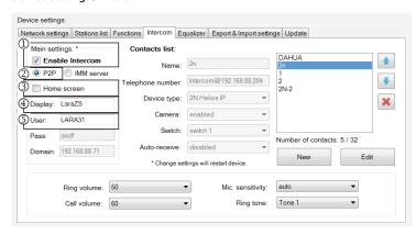
P2P - The Intercom function is used to make direct calls between devices using VOIP (Voice Over Internet Protocol) technology.
