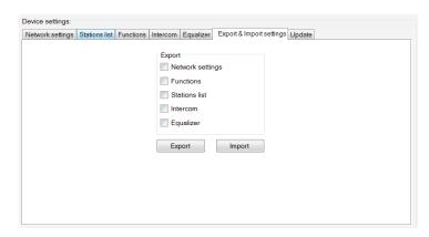
Export & Import settings: With these functions, you can easily back up and restore selected items - network settings, features, station list, intercom and equalizer. Created backups are in the\*.lcf format - backups of station lists from older firmware are not compatible with this system.
